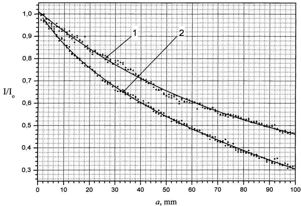
Figure 4: Relative SEW's intensity  $I/I_0$  visa distance  $a$  run by the SEW for clean aluminum surface (curve 1) and the surface covered with 100 nm germanium layer (curve 2).
