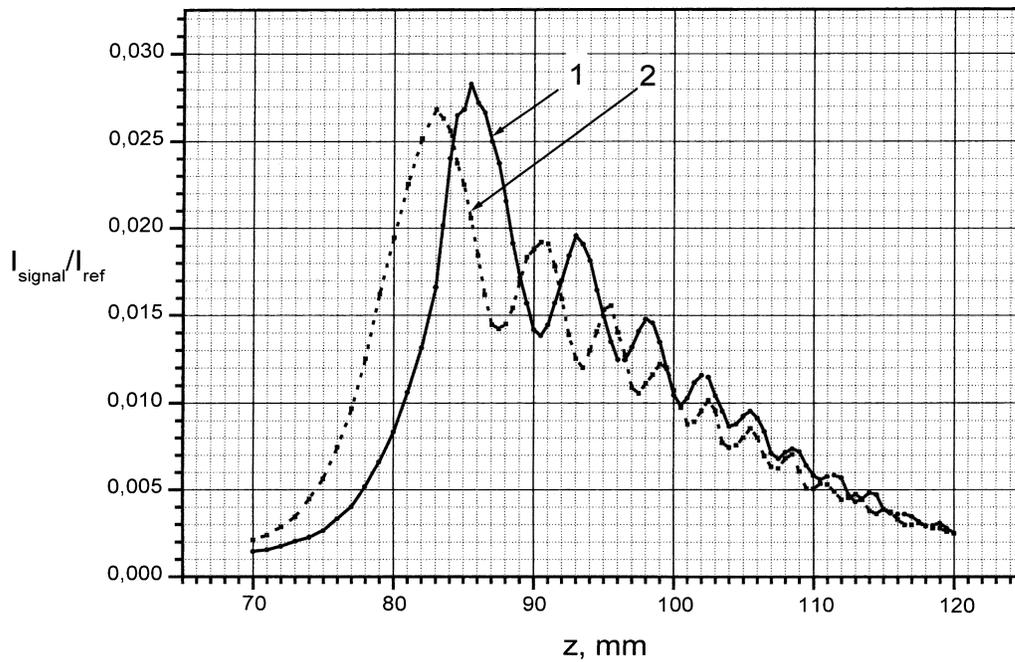
Figure 3: Interferograms obtained for clean aluminum surface (curve 1) and for the surface covered with 10 nm thick germanium layer (curve 2). Distance run by the SEW is  $a=120$  mm.
