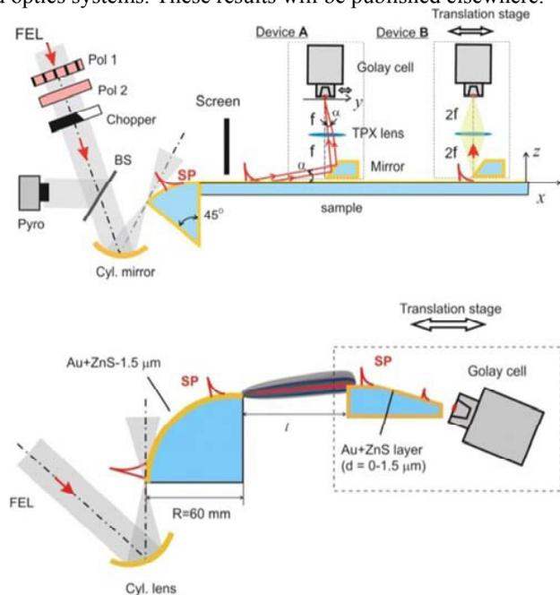
Fig. 5. Experimental setups for investigation of surface plasmon polaritons in the terahertz spectral range. Upper schematic: study of SPP propagation length, decay length and radiative loss; lower schematic: study of plasmon jumps between two metal-ZnS-air interfaces.
