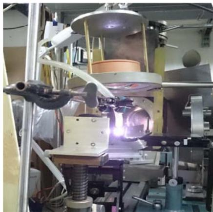
Fig. 4 Quasi-continuous optical discharge ignited by NovoFEL radiation in the focus of high-NA parabolic mirror;  $\lambda=130 \mu\text{m}$ .
