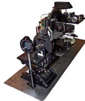
Fig. 9. General view of the ellipsometer designed for study of surfaces and films using tunable radiation of NovoFEL.
