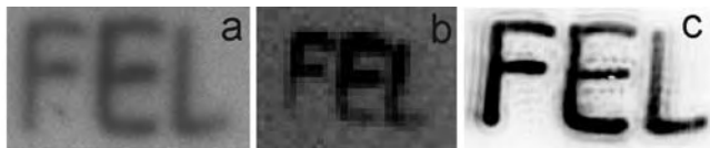
Fig. 2: IMAGES OF THE MASK FEL WITH - (a) The temperature sensitive phosphor plate, (b) the thermal recorder and (c) the microbolometer focal plane array.
