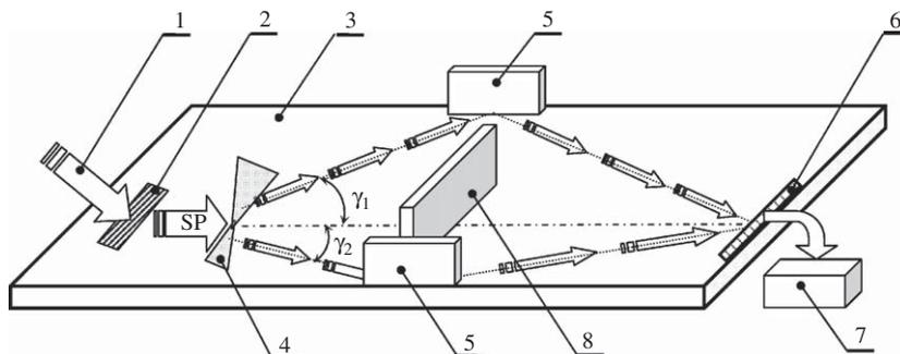
Fig. 4. THz SPs interferometer intended to measure the SPs refractive index and its changes: (1) bulk wave; (2) diffraction element; (3) specimen; (4) geodesic beam splitter; (5) plane vertical mirrors; (6) photo detector array; (7) computer; and (8) absorber of the bulk waves produced on the element 2.
