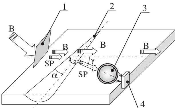
Fig. 3. Scheme of the THz SPs absorption sensor: (1) aperture; (2) geodesic prism; (3) geodesic lens; and (4) detector.
